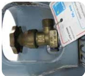
CO2 CON DISCO DE ROTURA ( a 80 Kg/cm<sup>2</sup> )
